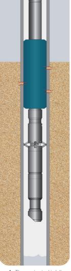
Stage 4 - The running tool is fully removed allowing the full filter section to expand to the damaged section. Anchors are locked in the casing and running tool is pulled out of hole.
