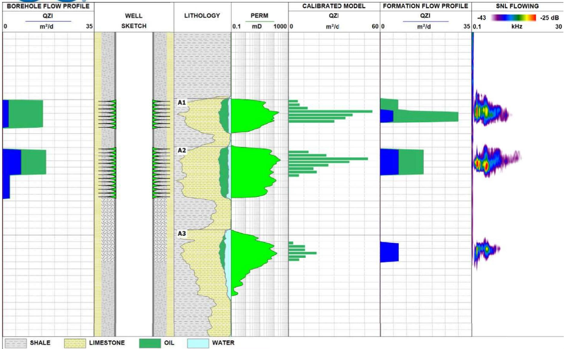
In reality, there was unwanted water production from the unperforated A3 Unit through behind-casing channelling.
