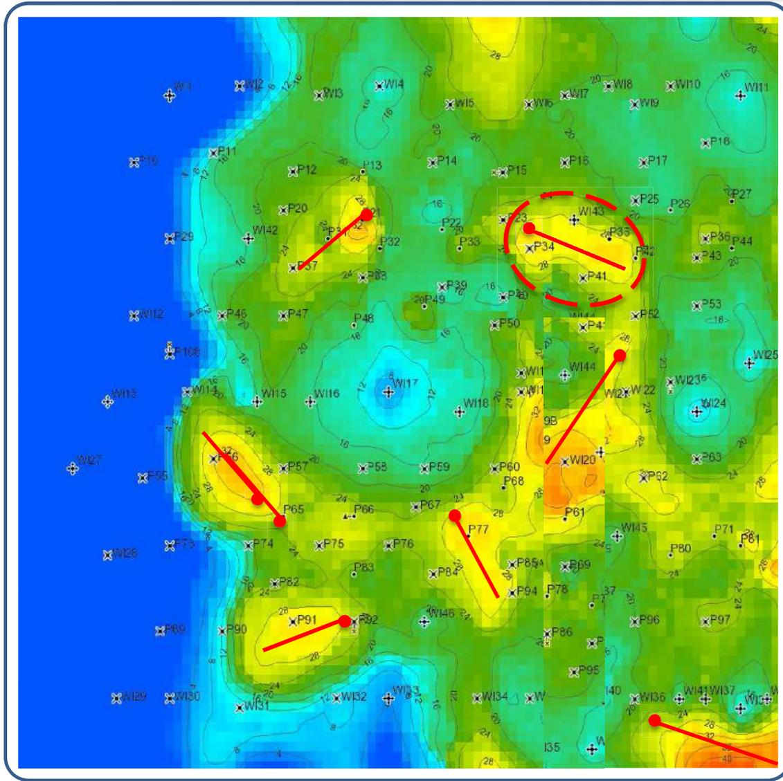
The calibrated model suggests that a sidetrack drilling plan should target bypassed and low-mobility oil.
