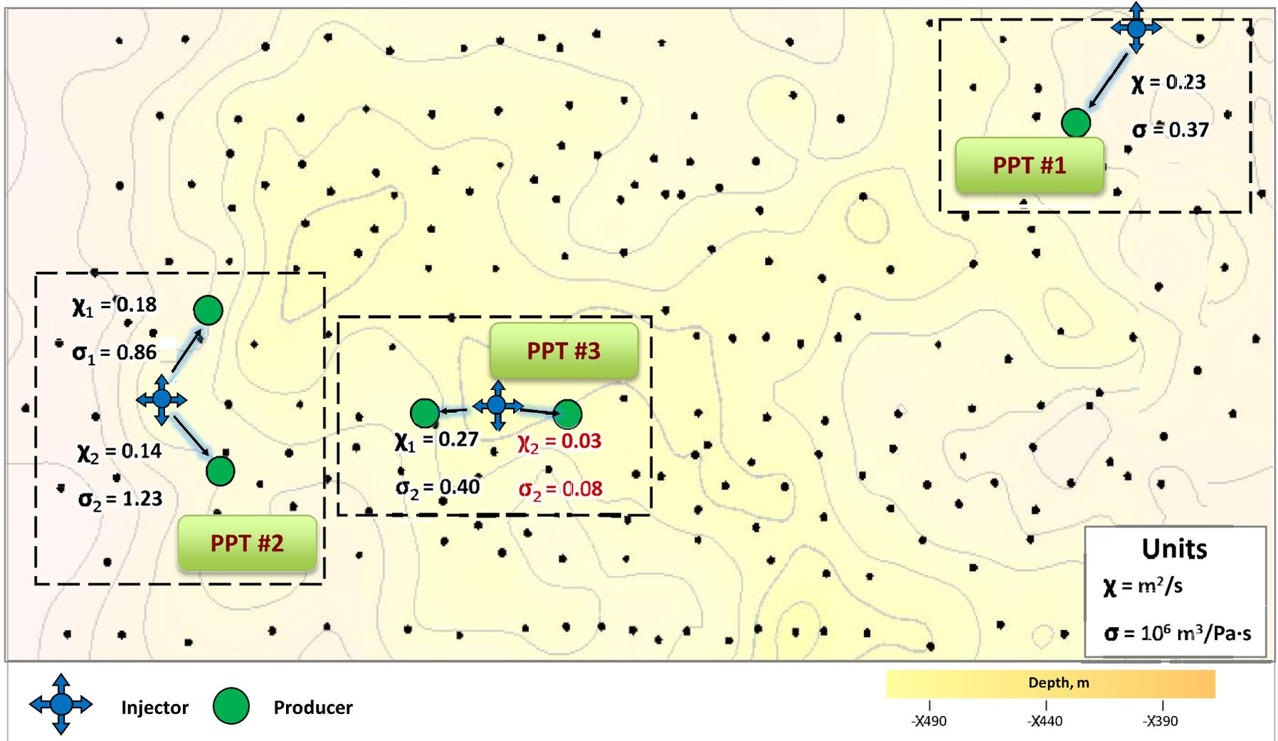
In this study, three pressure pulse tests were performed in aquifer and water-flushed areas in which the fluid saturation was known.
