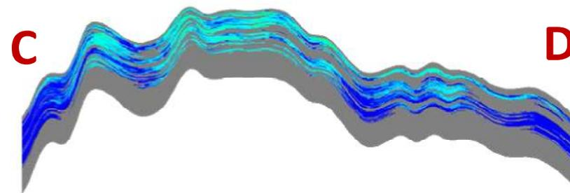
The study was carried out for a West Siberian oil field with a porosity ranging between 15% and 19% and high shale content. The permeability ranges between 15 mD and 50 mD. A core study found that water flooding can ensure 50% oil displacement efficiency. The field has been producing for almost 34 years with 610 producers and 255 injectors for pressure support. When the average water cut reached 95%, the recovery factor was 15% below expectations.
