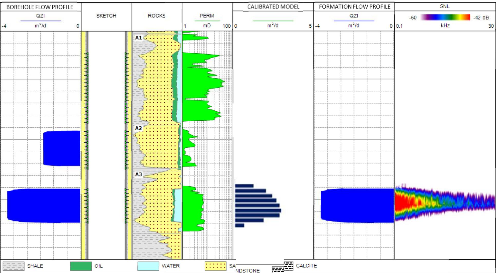
Unlike PLT, the HPT-SNL survey is reservoir-orientated, so it can see into the reservoir. In this case, it suggested that only the A3 Unit was flowing and that part of the flow was distributed behind casing through the A2 Unit perforations, which is captured by PLT but is misleading as to where this fluid came from. The actual reservoir flow profile is shown in the FORMATION FLOW PROFILE log data panel and a corresponding computer model is shown in the CALIBRATED MODEL log data panel.
