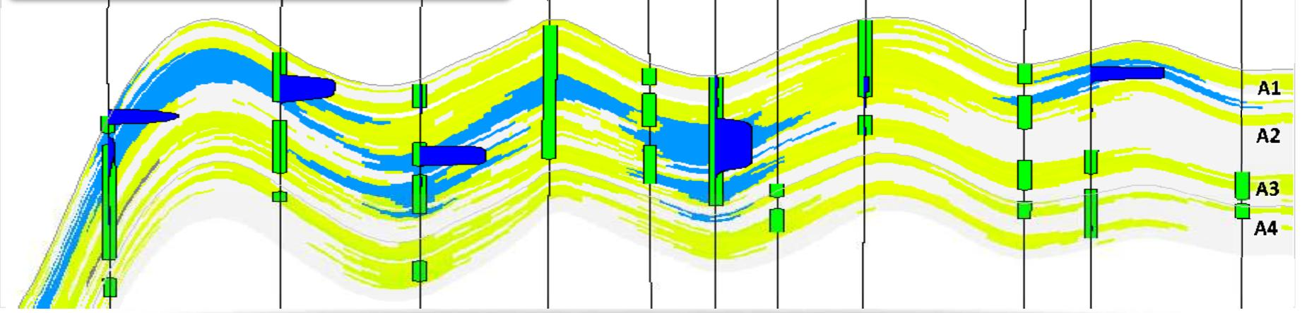
This cross-section illustrates the difference in residual oil distribution and displays bypassed oil zones. Note that injection flow dominates in the A3 Unit that apparently has better reservoir qualities relative to the overlying and underlying units. This led to short-circuiting in the A3 Unit and loss of flow circulation in other units with consequent 15% recovery delay.
