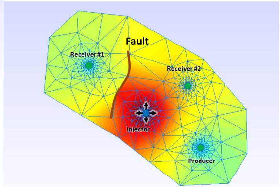
Cross-well interference testing is a powerful reservoir characterisation technology.
