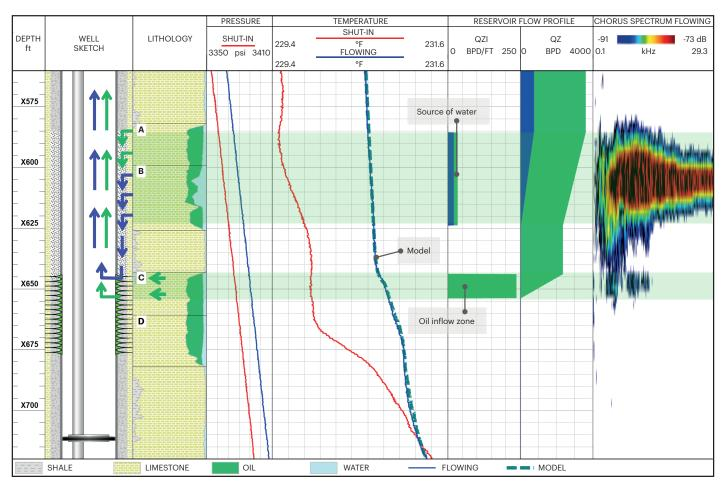
Behind-casing crossflow from upper unperforated units.
